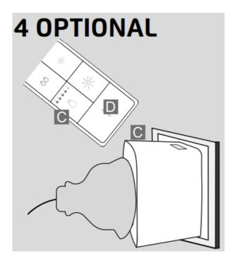
To operate the ZCC-3500 only with the ZYCT-202, follow steps C and D from chapter 5. **Note:** Make sure the switch is not in connection mode (LED flashes slowly). Stop the connection mode by briefly pressing the button on the housing. The LED on the switch stops flashing. After this follow steps C and D from chapter 5.
