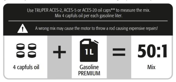
To prolong the useful life of the motor use TRUPER two-cycle synthetic motor oil. \* 1
