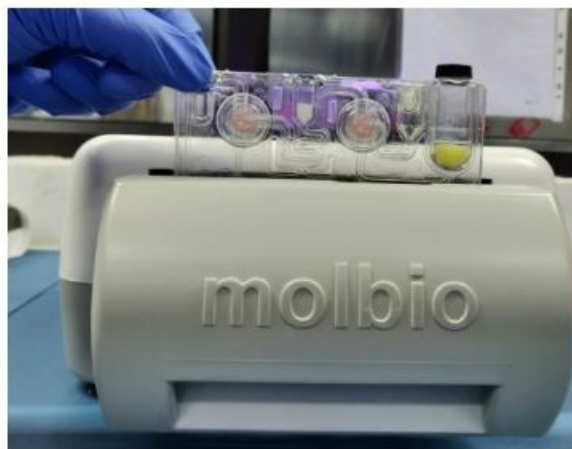
Figure 11: Cartridge being placed in cartridge holder
