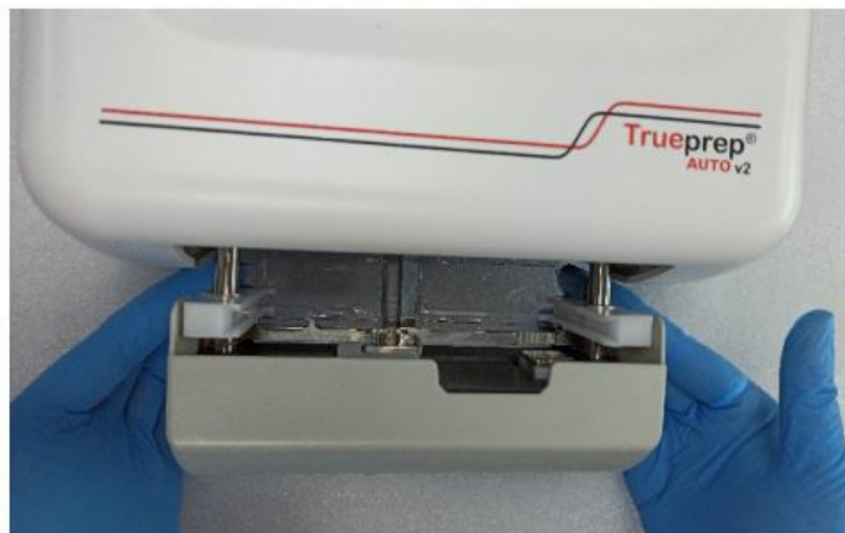
Figure 15: Replacement of discarded Replaceable tray with new
