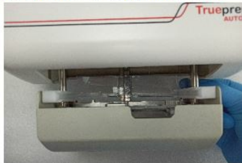
Figure 14: Removal of Replaceable Tray from cartridge holder
