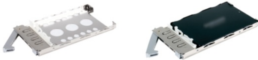
48 SSD drive trays with up to 48 drives installed
