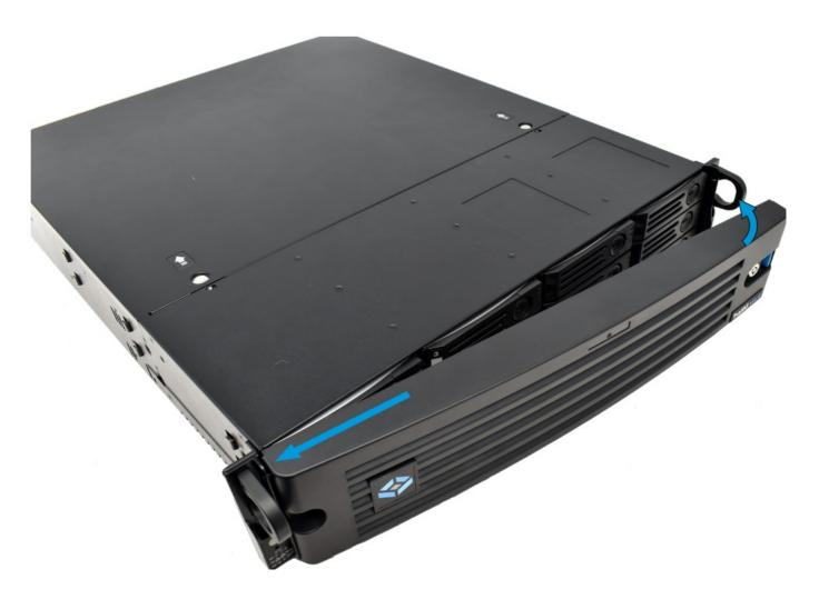
You can lock the bezel for added security. To do so, insert a key in the lock and turn it ninety degrees clockwise.
