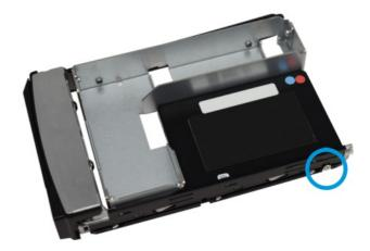
Use three HDD screws to attach the adapter and SSD to the drive tray.
