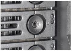
For extra security, you can lock the drive tray into the system. The tray button is unlocked when the inner slot is horizontal and locked when the slot is vertical. To lock a tray, insert a flat-head screwdriver into the center button slot and gently turn it ninety degrees clockwise until the slot is vertical.
