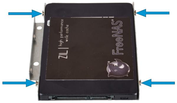
Replace the tray on the chassis by aligning the tray retention clips with the holes in the chassis, sliding the tray into place, and reattaching the original screws. Repeat the process if a second SSD is being installed.
