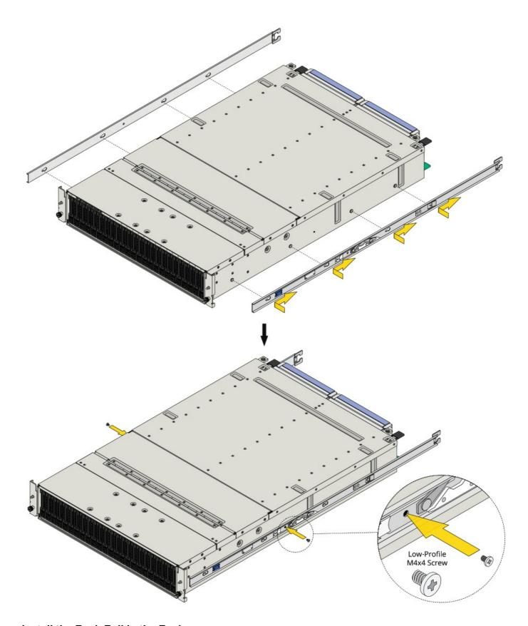
Install the Rack Rail in the Rack
