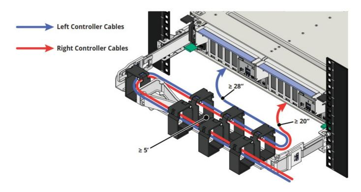
Connect ethernet network cables from your local switch or management network to the Out-of-Band Management (OOBM) and TrueNAS Management ports on both controllers.
