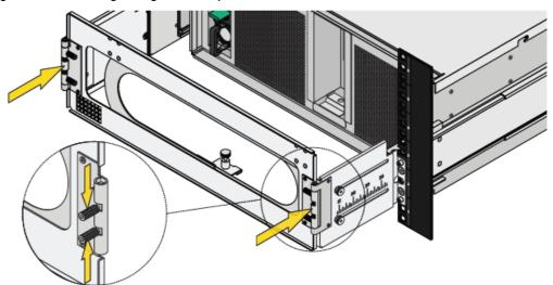
Pull the CMA attachment pin up and move the pin assembly toward the CMA attachment bracket on the chassis. Fit the pin assembly lip over the CMA attachment bracket on the chassis, then pull it back and release the pin to lock the CMA to the system chassis.
