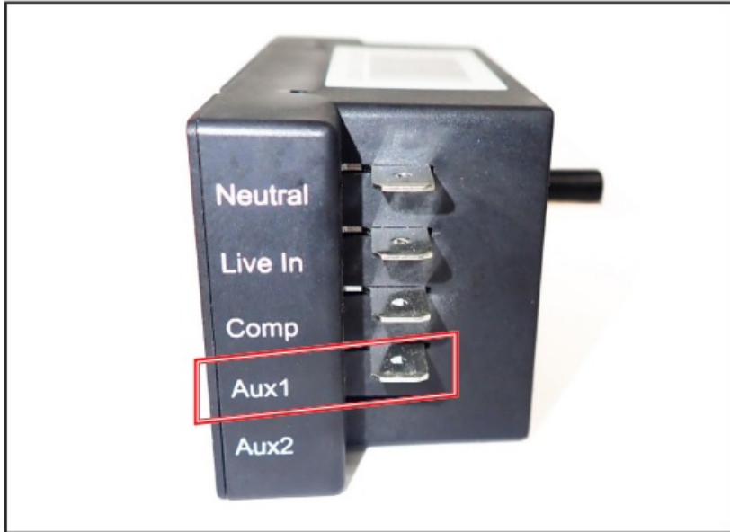
Fig. 3. Aux1 terminal of the replacement electronic temperature control.
