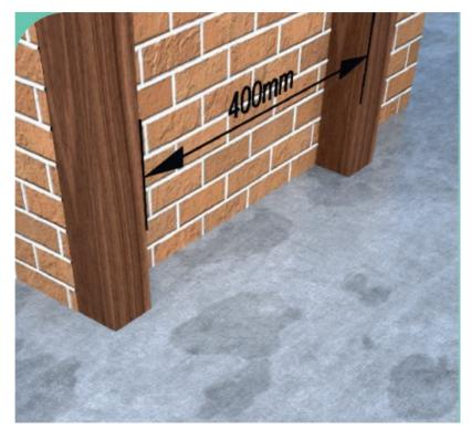
Install wooden / aluminium or composite battens to desired area at 400mm centres.
