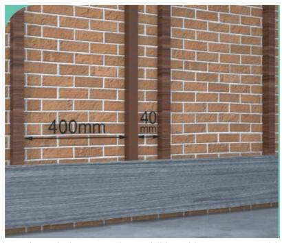
2. Please ensure where boards butt together additional battens are added as per photo.
