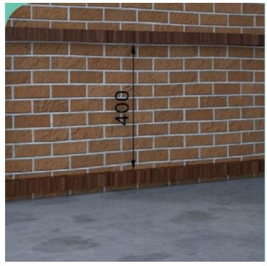
Install wooden / aluminium or composite battens to desired area at 400mm centres.
