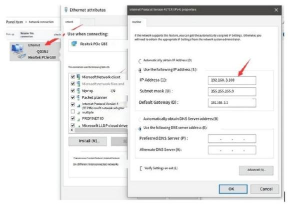
2. Step 2: Open the network assistant, select the TCP client, enter the remote host IP192.168.3.7 (default parameter), enter the port number 502 (default parameter), and select HEX to send.
