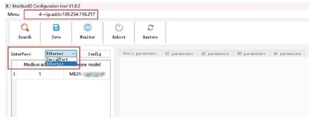
2. If you choose a serial port, you need to select the corresponding serial port number, and the same baud rate, data bit, stop bit, parity bit and address segment search range as the device, and then search.
