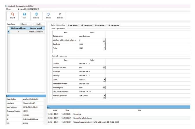
3. Step 3: After configuring the parameters, click Download Parameters. After the prompt message in the log output shows that the parameters are saved successfully, click Restart the device. After the device restarts, the modified parameters will take effect.
