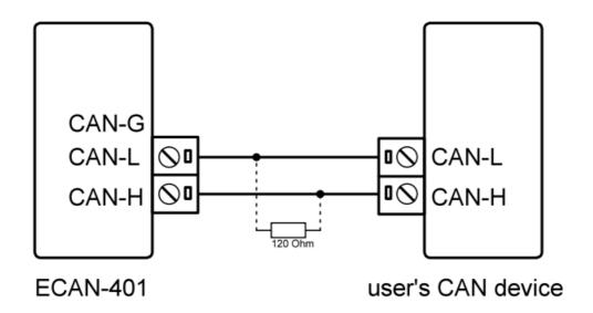
The linear topology is the most commonly used in the CAN bus wiring specification. That is, the two lines of the main trunk branch out branch lines to each node. Both ends of the backbone are equipped with suitable terminal resistors to achieve impedance matching (usually 120 ohms within 2km).
