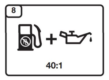
Mix thoroughly in a separate fuel can: —  $3.2 \, \text{fl.}$  oz. of 2-cycle engine oil —  $1 \, \text{gallon}$  of fresh unleaded gasoline (less than  $30 \, \text{days}$  old)
