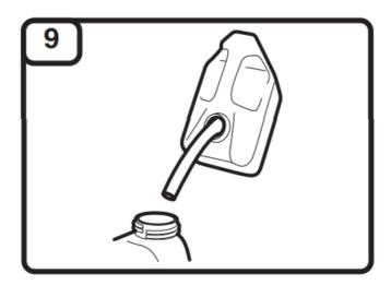
Position the unit with the fuel cap facing up. Slowly remove the fuel cap. Fill the fuel tank. Reinstall the fuel cap. Move the unit at least 30 ft. (9.1 m) from the fuel container and the fueling site before starting the engine.
