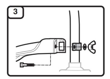
Insert the square bolt into the hole underneath the cutting head shield. Push the square bolt through the cutting head shield and mount bracket. Place the washer and wing nut onto the square bolt. Tighten the wing nut securely.
