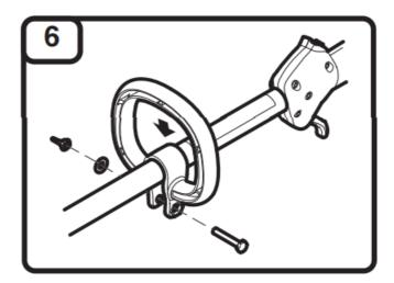
Push the handle down onto the upper shaft housing. Make sure the hex hole faces left. Insert the bolt into the hex hole. Place the washer onto the bolt. Screw the wing nut onto the bolt, but do not tighten it completely.
