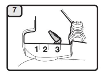
START: Move the choke lever to Position 3.
