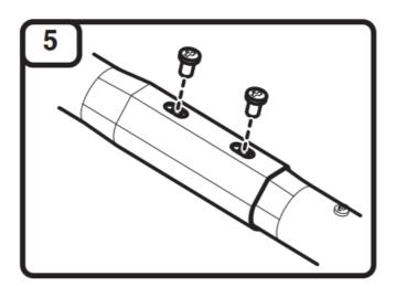
Insert the screws (x2) into the aligned holes. Tighten the screws securely with a #2 Phillips screwdriver.
