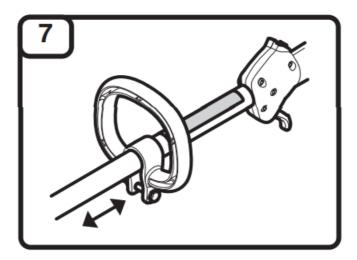
Move the handle to a comfortable location. Make sure the handle is positioned beyond the end of the safety label. Tighten the wing nut until the handle is secure.
