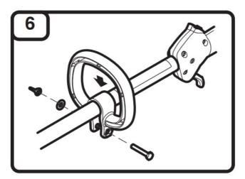
Push the handle down onto the upper shaft housing. Make sure the hex hole faces left. Insert the bolt into the hex hole. Place the washer onto the bolt. Screw the wing nut onto the bolt, but do not tighten it completely.
