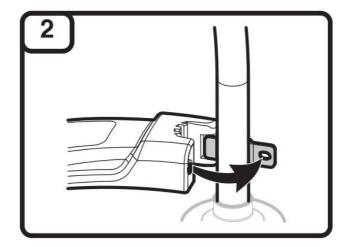
Insert the short tab (the one without a hole) on the mount bracket into the slot on the cutting head shield. Rotate the cutting head shield counterclockwise.
