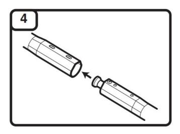
Push the lower shaft housing into the coupler. The holes on the lower shaft housing should align with the holes on the coupler.
