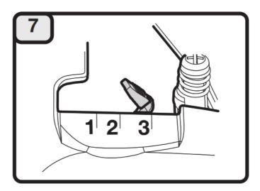
Move the handle to a comfortable location. Make sure the handle is positioned beyond the end of the safety label. Tighten the bolt until the handle is secure.
