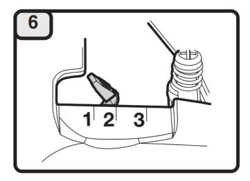
Push the handle down onto the upper shaft housing. Make sure the bolt hole faces to the right. Insert the bolt into the bolt hole. Tighten the bolt with a flat-head screwdriver, but do not tighten the bolt completely.
