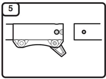
Align the release button with the guide recess. Push the attachment straight into the coupler until the release
