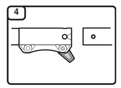
Remove the hanger cap from the attachment. If present, remove the gray spacer from the coupler. Turn the knob counterclockwise to loosen the couple
