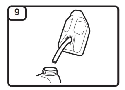
Position the unit with the fuel cap facing up. Slowly remove the fuel cap. Fill the fuel tank. Reinstall the fuel cap. Move the unit at least 30 ft. (9.1 m) from the fuel container and the fueling site before starting the engine.
