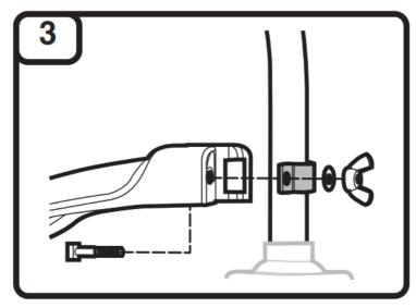
Insert the square bolt into the hole underneath the cutting head shield. Push the square bolt through the cutting head shield and mount bracket. Place the washer and wing nut onto the square bolt. Tighten the wing nut securely.
