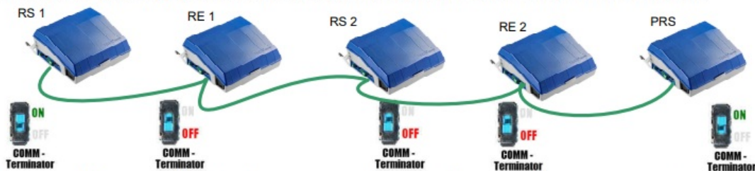
Example 4: Three supply air with one exhaust air controller, one duct pressure and one room pressure controller
