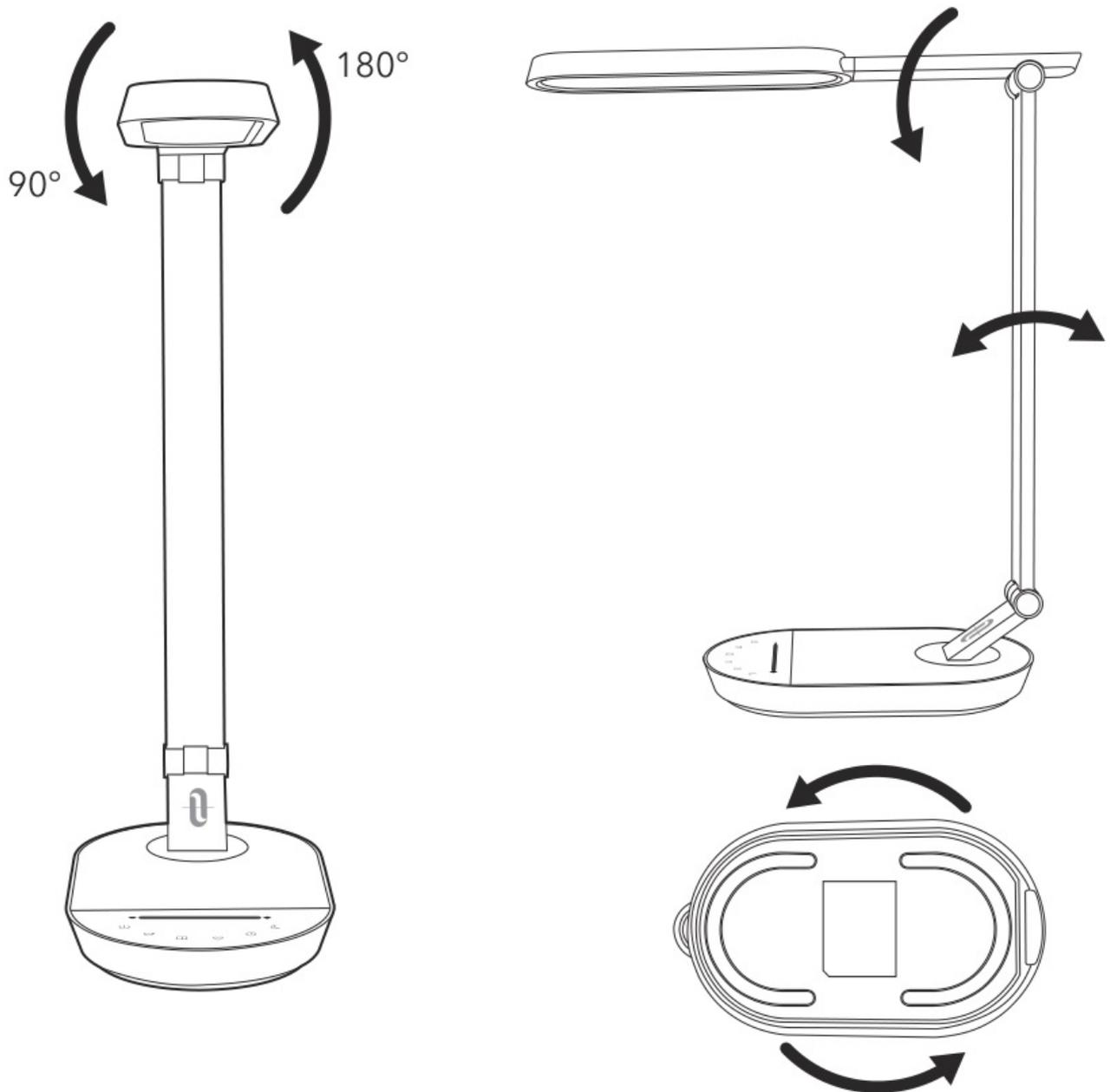
The lamp head is 90 degrees rotatable to the left and 180 degrees to the right.
