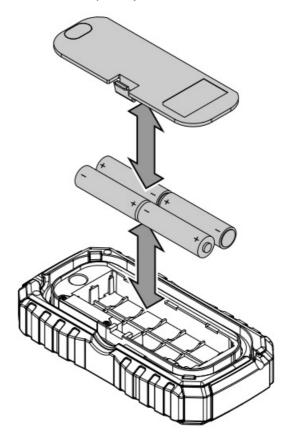
3. Put the cover back onto the battery compartment.
