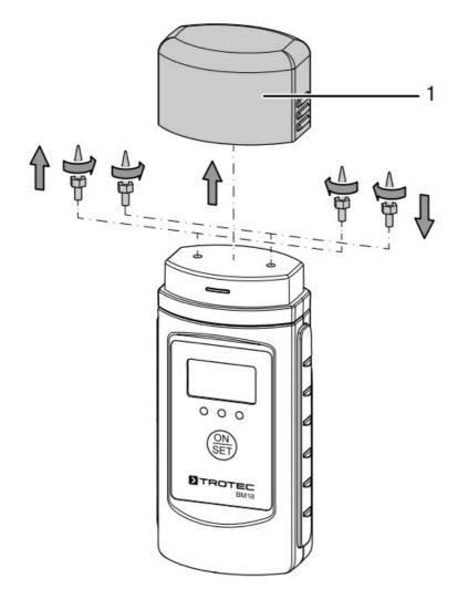
3. Screw the new measuring tips into the device.
