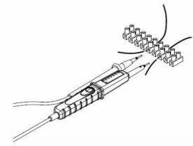
• The LED display (2) is illuminated according to the existing voltage.
