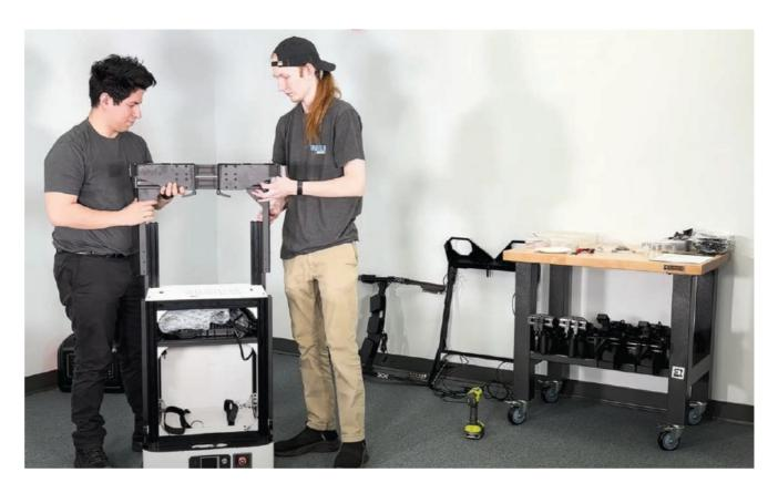
**TIP:** When loosening the locks or adjusting the height of ViperX or WidowX Vertical Mounts, be sure to hold the assemblies so that they do not fall. It is highly recommended that you use a second person to hold them in place.
