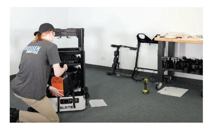
**TIP:** Place the power station next to the opening and put the top velcro straps through the handle before picking the power station up and placing it into the podium.
