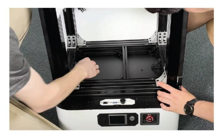
**TIP:** If a bolt is not threading into its intended hole easily, loosen other bolts in the same bracket/plate and reposition as needed. Any Loosened bolts will require fresh loctite.
