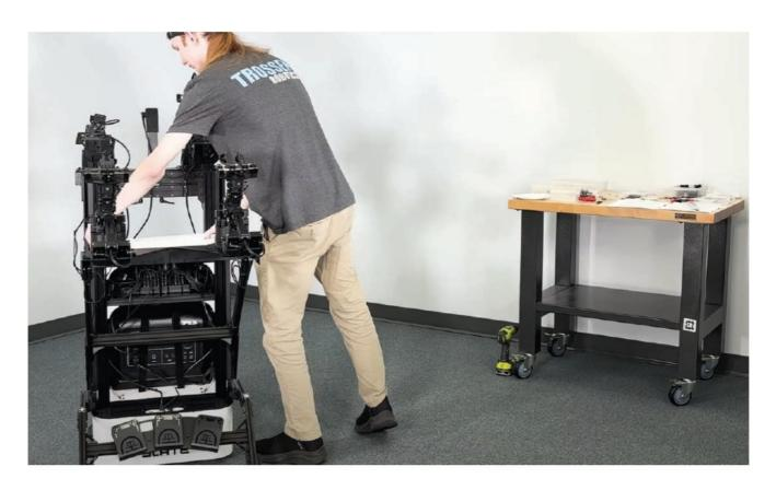
**STEP 23**Secure the connected cables to the underside of each arm.
