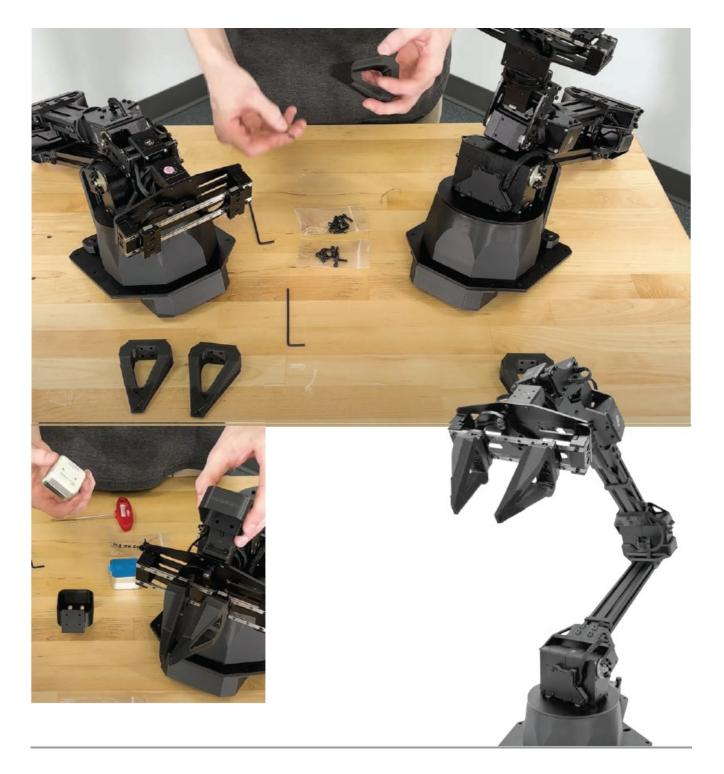
Add ViperX arms onto front follower arm mounts M5x10b using Loctite. Don't let go of the ViperX until two bolts are screwed in.
