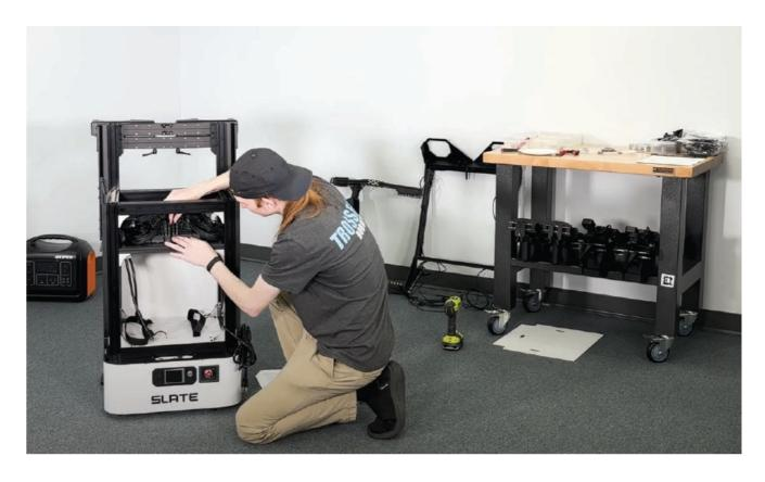
Insert power station into podium. Secure the power station with Velcro straps. Connect the 1ft outlet extensions to the top 2 outlets, and add the 4-outlet power strip cord into the bottom outlet.
