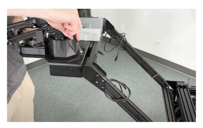
Add micro USB-B locking cables to hubs, and zip tie to the electronics shelf to avoid damaging electronics in case cables catch on anything. Attach micro USB-B into cameras. Use 2040 cable clips for cable management.
