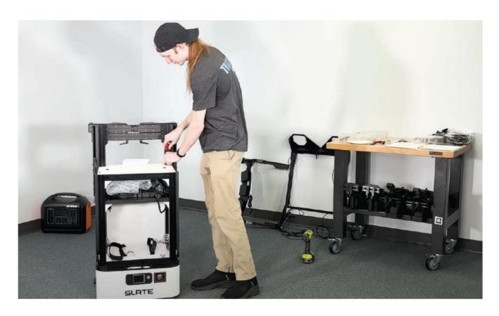
**STEP 8**Check all power supply cable connections and all USB cables in the USB hubs. Confirm that all buttons corresponding to used USB ports are pressed down.
