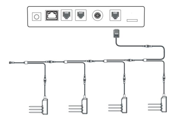
When connecting multiple WCS-3 to the TrolMaster controller, it is recommended to use one or more of the SPH-1 splitter hubs to power and connect the WCS-3 sensors. The SPH-1 has 8 separate RJ12 connection ports and each SPH-1 can power up to 20 WCS-3 sensors. Up to 5 WCS-3 can be connected to a single RJ12 port on the SPH-1. The SPH-1 then connects to the appropriate RJ12 port on the TrolMaster controller to integrate all of the connected WCS-3.
