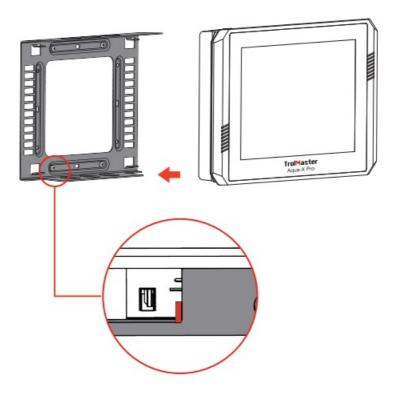
3. Slide the controller from right to left until it "locks" into place.
