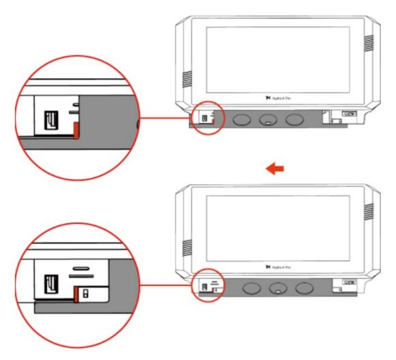
4. To release the controller, press on the lock and slide the controller to the right.
