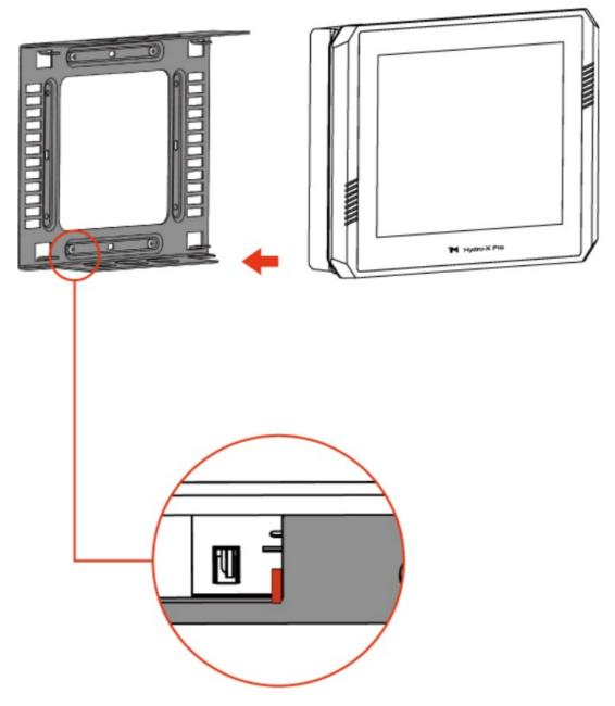
3. Slide the controller from right to left until it "locks" into place.
