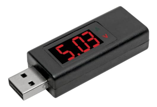
Measures, tests, and monitors the voltage and amp capacity of your computer or laptop's USB ports and any
