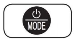
**ON/OFF/MODE Button:** Press and hold for 2 seconds to turn on the UPS and 2.5 seconds to turn the UPS off. When the UPS is on, tap this button repeatedly to advance through LCD screens. If utility power is absent, pressing and holding this button for 2.5 seconds will "cold-start" the UPS; i.e. turn it on and supply power to the outlets from its batteries.
