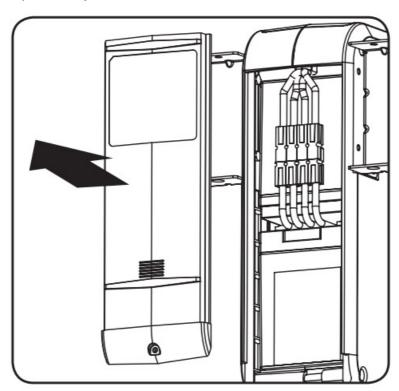
3. Disconnect the positive (red) and negative(black) connectors and carefully remove the old battery from the unit.
