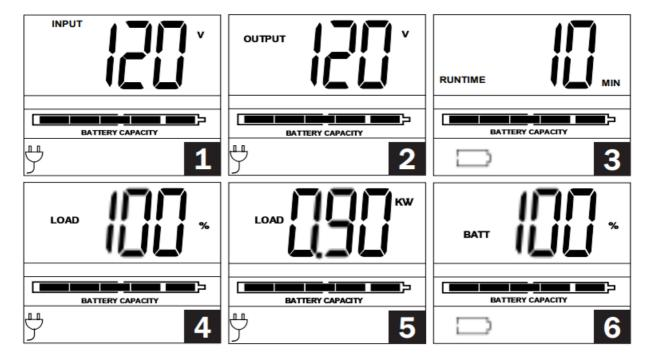
Load Wattage is displayed in watts up to "999", and then will be displayed in Kilowatts.
