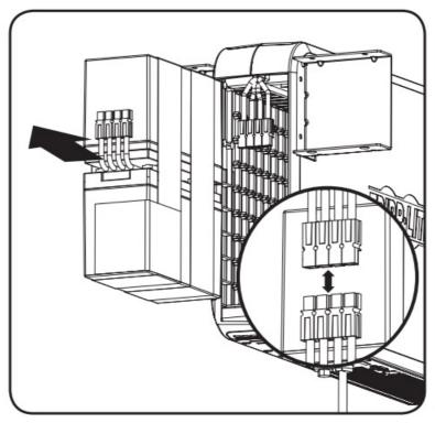
4. Carefully place the new batteries into the UPS and connect the positive (+) (red) connectors and negative (-) (black) connectors.
