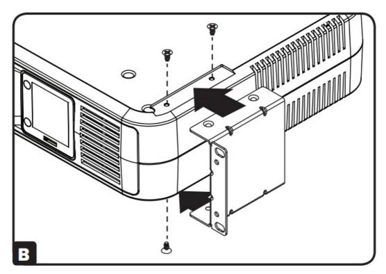
**CAUTION**: If the UPS is installed in a rack, allow at least 2 cm (0.75 in.) clearance above and below the unit. If the UPS is placed on a flat surface, do NOT stack any other object directly on top of the unit.
