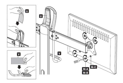
**Warning:** Please make sure you attach identical monitors to the table stand; otherwise, the table stand might be inverted. Also, while you are installing a monitor on one side, another person should hold the other side of the mount to keep the table stand stable. Use an assistant or mechanical lifting equipment when hooking the display onto the mount and fastening the screws as shown. Firmly secure all screws. Do not over-tighten.
