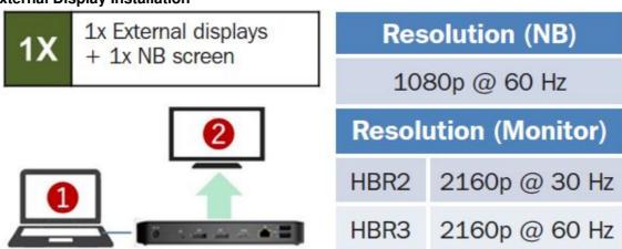
**A.** Connect an HDMI or DisplayPort cable (see Optional Accessories) between the U442-DOCK8-B and a compliant display.
