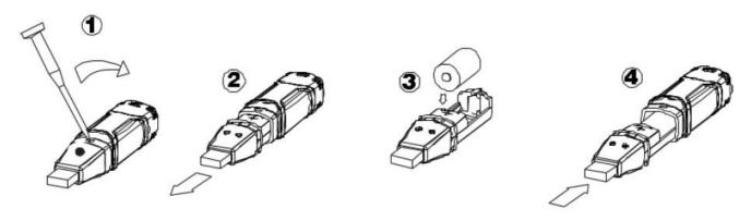
**WARNING:** Handle lithium batteries carefully, observe warnings on battery casing. Dispose of in accordance with local regulations. Safety: Please dispose of batteries responsibly; never dispose of batteries in a fire, batteries may explode or leak. If the meter is not to be used for 60 days or more, remove the battery and store it separately.
