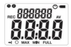
**REC:** Recording status. After the record mode is set up by the software, press the START/STOP button for more than 4 seconds to begin recording. This icon will be displayed and indicates the meter is recording data. Press the same button again for more than 4 seconds to stop recording.
