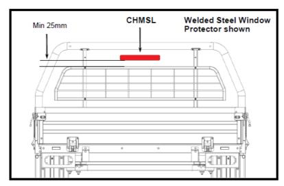
Fasten the window protector to the head-board uprights upright using M6x40 counter sunk screws and M6 nyloc nuts.
