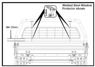
If the vehicle is fitted with a CHMSL (Center High Mounted Stop Lamp) ensure the top of the window protector sits 25mm below the bottom of the lamp. The brake light must not be blocked by the window protector. Mark the hole locations on the headboard uprights and drill 6.5mm holes.
