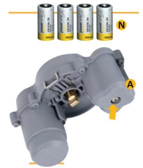
Inserting batteries in the Actuator Remove the plastic wrap from the batteries **N**. Using a Phillips screwdriver, open the battery to the compartment located on the bottom of the Actuator **A**. Note the correct direction for their insertion to the cell; all should be facing the same direction. Close the compartment again with the Phillips screwdriver.
