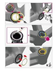
Carefully press the seals back into place on the bearings, ensuring they are seated properly and
