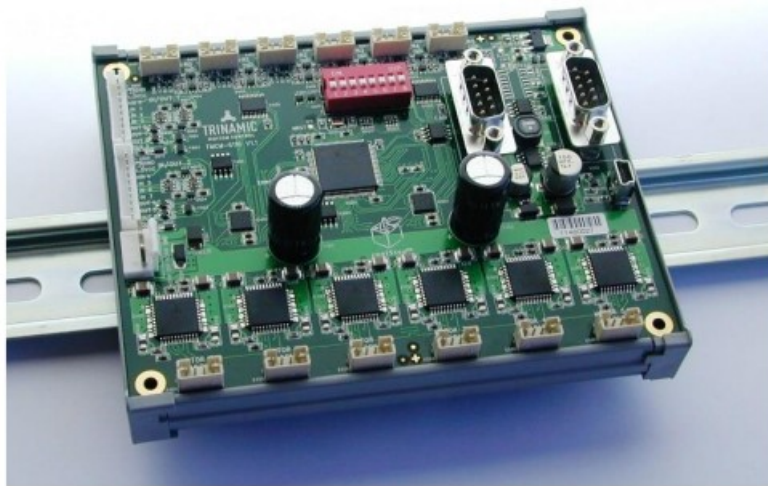
Figure 3.2 DIN rail mounting
