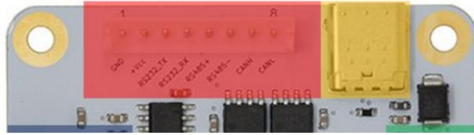
Figure 3: Power / communication connector of TCM-0960-MotionPy V21
