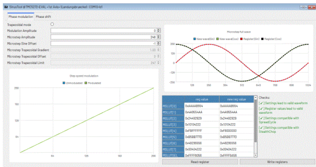
Figure 18: Configuring and read out the sinus and phase shift registers of a TMC5272 (similar for other ICs).
