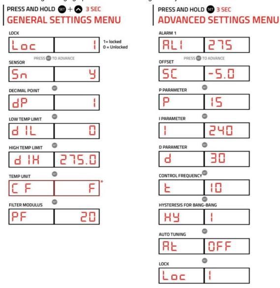
**NOTICE** Make sure your Temp Unit is set to Fahrenheit. Setting Fahrenheit temps in Celsius can result in melting components of the machine.
