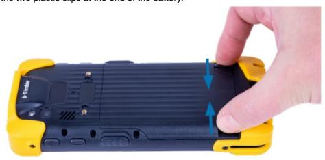
2. Push the battery forward and lift to remove it.
