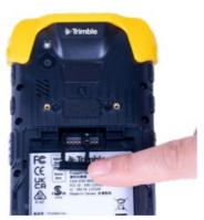
2. The card holder can hold two nanoSIM cards, or one nanoSIM card and one microSD card at a time. Insert your cards as needed, as follows:
