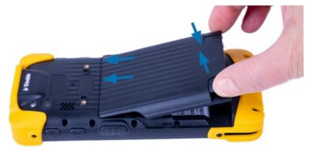
3. Press the battery down to secure it in place.
