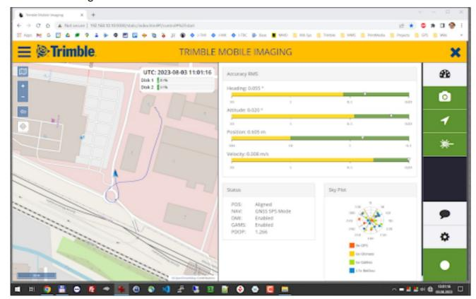
**NOTE** – Depending on your working environment, the time period can vary for the system to resolve its ambiguities, so it is advised to add some time (up to 10 minutes) before logging data to avoid poor results at the start of recording runs.
