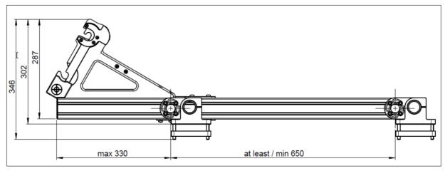
4. Attach the screw bridge and tighten all screws on the MX SCAN Roof Rack.
