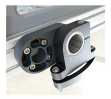
The distance from the back brackets to the end of the MX SCAN Roof Rack must be a maximum of 330 mm. The minimum space between mounting brackets must be 650 mm.
