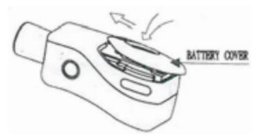
5. Examine: After the lock is locked if there is a sound "DI".it shows you correctly installed the battery. If without the sound "DI", please reinstall the battery according to the 4 steps
