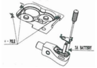
4. Press the battery cover as the drawing shows and move ahead to the battery cover.
