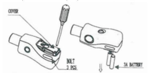
3. Install the battery according to the "+-" pole and rotate the bolt tightly. Attention: You should rotate the bolt tightly in order to prevent the water from flowing to the lock body to damage the alarming system
