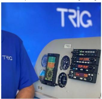
Dual Watch allows the monitoring of a second Com frequency – this is something that once you have tried, you really don't want to give up! For example, It's useful when listening to ATIS on the secondary frequency and monitoring ATC on the primary frequency. The primary frequency always takes precedence, so you really can communicate and monitor at the same time. Dual Watch is also possible on the Nav – making VOR navigation more accurate by generating a second position fix if desired.
