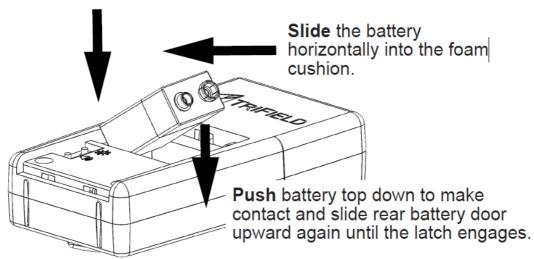
Replace the battery when the battery level icon in the upper right corner of the LCD drops to zero bars. Typical
