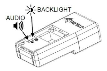
Audio and light buttons are located in the battery compartment. While the meter is on, you can press these green buttons to turn the backlight on or off and to turn the audio option on or off.
