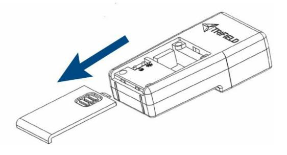
• Insert the bottom of the battery into the center of the compartment at an angle.
