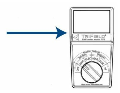
• For both Electric (ELEC) & Radio (RF) field measurements, hold the bottom half of the meter below this point. Do not block the top of the meter with your hand. Point the meter outward, away from your body. The reading may be higher when holding the meter than if it is set down. This is because the body concentrates the field. Therefore, hold the meter to get a true reading of your full exposure.
