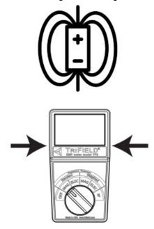
For both Electric (ELEC) and Radio (RF) field measurements, hold the bottom half of the meter below this point. Do not block the top of the meter with your hand. Point the meter outward, away from your body. The reading may be higher when holding the meter than if it is set down. This is because the body concentrates the field. Therefore, hold the meter to obtain a true reading of your full exposure.
