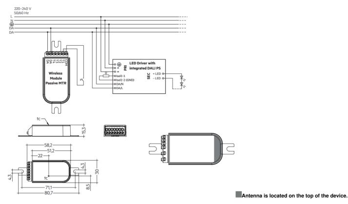
The Wireless Module Passive MTR is a Matter-capable DALI controller with 4 freely configurable push-button inputs. The module is supplied via the DALI bus, an additional mains supply is not required.
