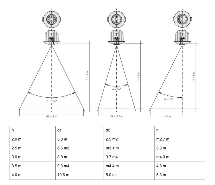
basicDIM Wireless Sensor provides movement detection and lux control wireless to other basic DIM Wireless devices to achieve smart control as presence detection or daylight harvesting.
