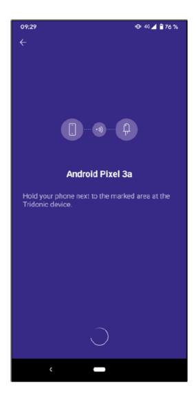
Now hold your phone or the NFC reader next to the marked area on the driver. The phone will vibrate when a connection is established. Wait for a few seconds until the driver has been read-out successfully.
