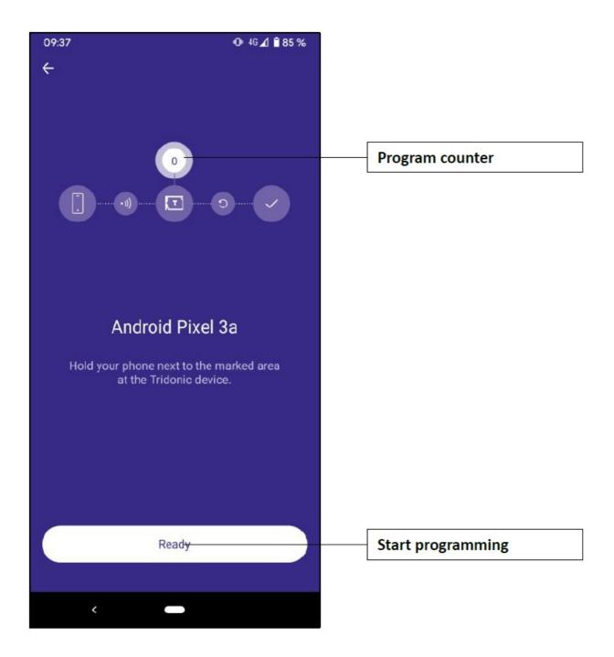
After the writing is finished, the counter on the screen will increase and you get the option to either verify the programming on the driver or to program another driver.
