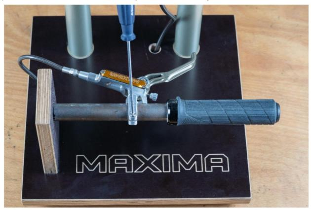
4. Use an 8mm open-end wrench to remove the brake hose from the brake pump.
