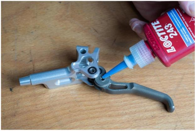
9. Before mounting the dial back onto the piston rod, make sure to apply a medium thread locker to this connection as well. Use a 7mm open-end wrench for tightening.
