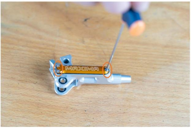
7. Lastly, remove the bleed bolt using a TX10 key. Dispose of the old O-ring and put a new one on.
