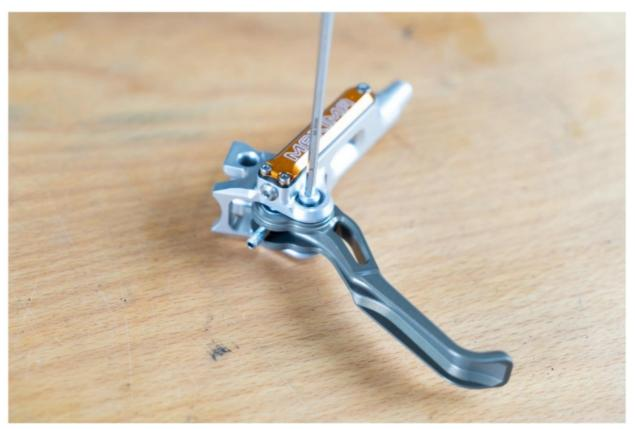
3. Use a HEX2mm key to remove the lever blade from the piston rod. Use a shop towel to clean the lever blade and put it aside, further service on the lever blade is not necessary.
