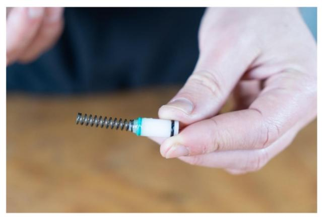
4. Push the pump piston into the pump housing. This should show only minimal resistance.
