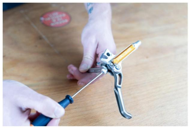
2. Remove both pivot bolts (upper and lower) using a HEX3mm key.
