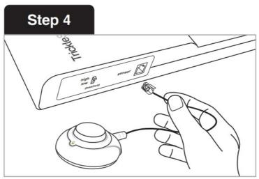
Plug the SensorClick timer footswitch into the port on the side of the power strip that looks like a phone jack and is marked "sensor".
